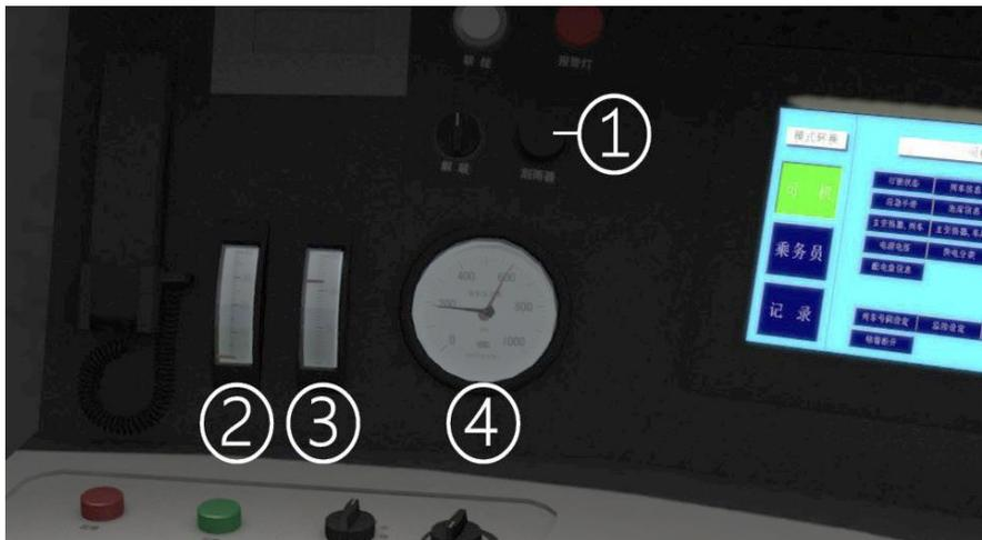
1 Wiper control 2 Traction voltage 3 Control system voltage 4 Pressure gage
