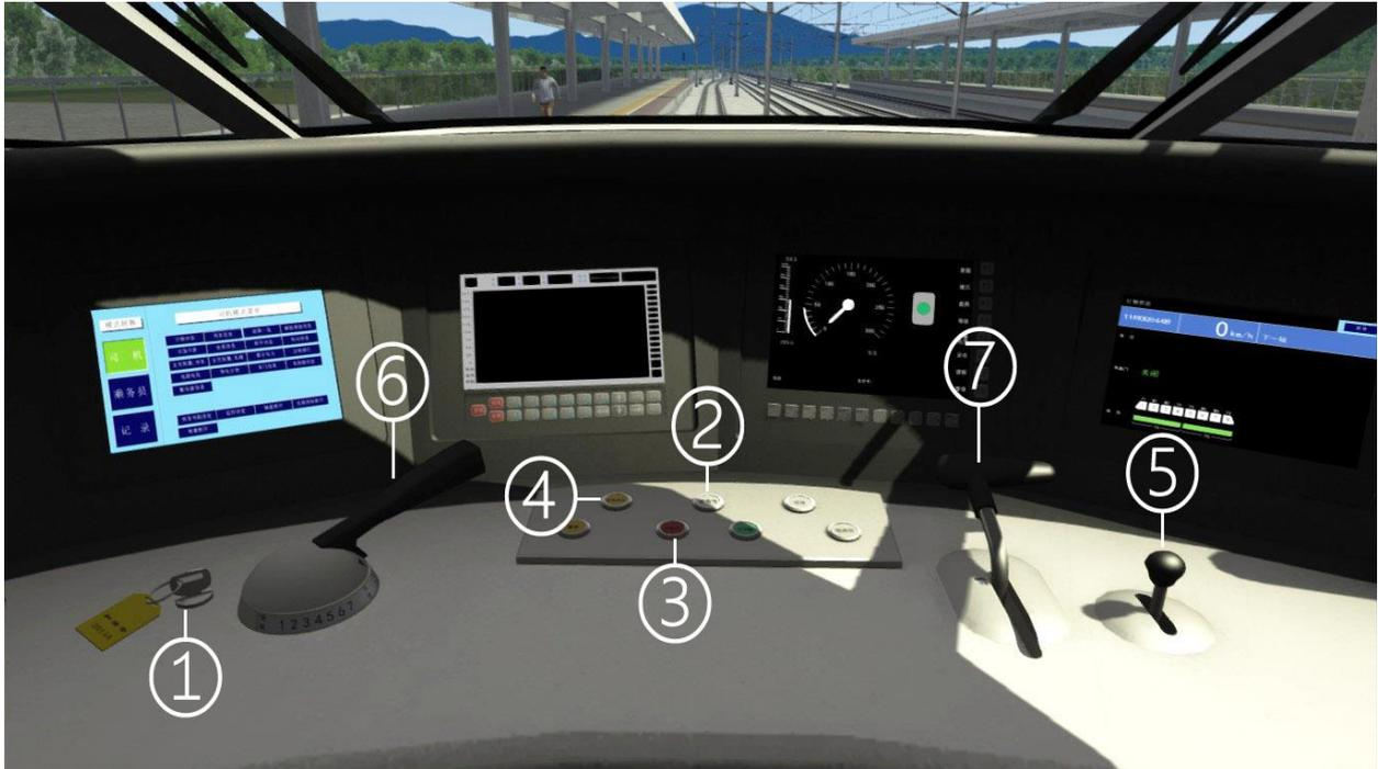
1. Turn the key to get the power on, so that the screen turns on and the control voltage shows 120 V.
