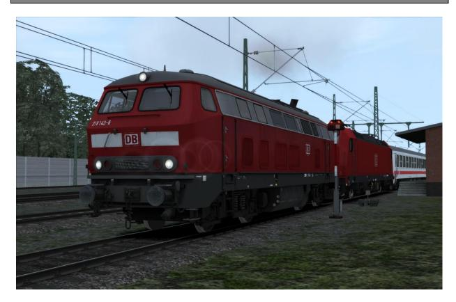
The DB BR218 (before 1968 the DB BR V 164) are a class of 4 axle, diesel hydraulic locomotives acquired by the Deutsche Bundesbahn for use on main and secondary lines for both passenger and freight trains.
