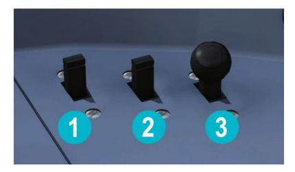
PZB controls on the Cab Desk of a BR474 (other locomotive controls would be similar but not identical)
