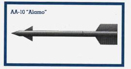
Nation of Manufacture: USSR Guidance: Semi-active radar-homing (requires radar guidance from plane) Effective Range: 82 km Missile Speed: Mach 3.5 Maneuverability: Fair Attack Technique: Semi-active radar-guided from launching aircraft Nationality and Aircraft: Soviet MiG-31s
