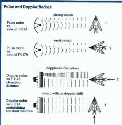
Figures 1 and 2 illustrate an F-117A reflecting pulse radar. When the F-117A has a low signature, the return can be so weak that he plane is "visible" to the radar. Note that the radar power varies, so the F-117A might be "visible" to a more powerful radar at that range. Power also varies with range, so the F-117A could become visible to either at a short range.
