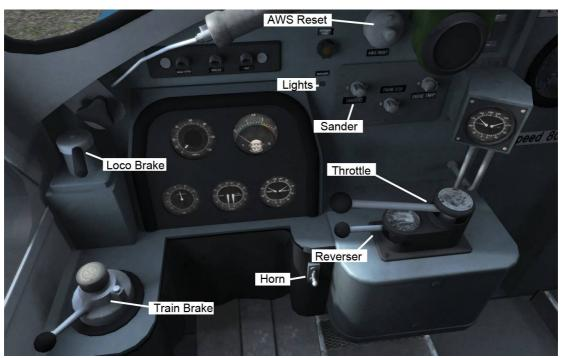
The diagram above shows the main controls of the Class 37.
