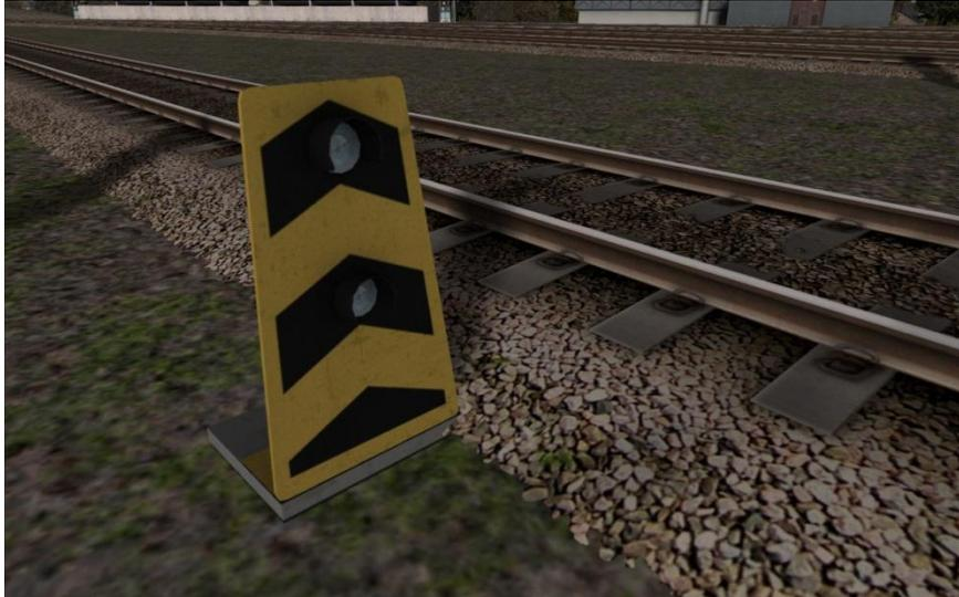
**Temporary AWS Magnets** – Temporary AWS magnets are used to warn drivers of a proceeding temporary speed restriction or of an emergency indicator board. Temporary AWS magnets are bi-directional.
