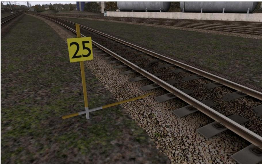
**Temporary Speed Restriction Boards (Interactive Objects)** – This board indicates that the temporary speed restriction has now been terminated and you can return to normal line speeds.
