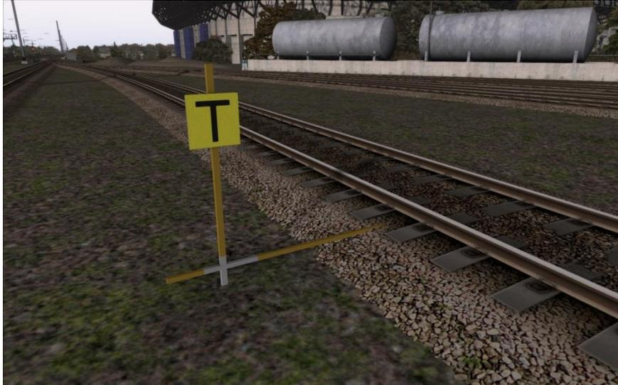
**Temporary Speed Restriction Boards (Interactive Objects)** – This board indicates that the AWS magnet beforehand does not apply to you.
