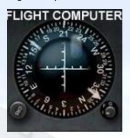
The F-89 had a unique predecessor to today's "Flight Director". It was called a "Flight Computer" and allowed a similar combination of gage functions to be incorporated into a single unit. We have recreated a facsimile of the Flight Computer which works in a similar way to the original.
