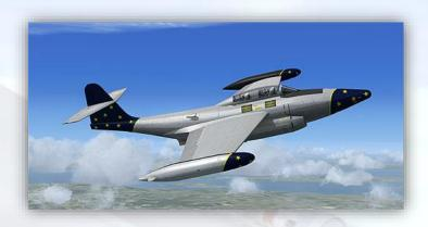
F-89D – wingtip rocket pods, underwing aux. fuel tanks
