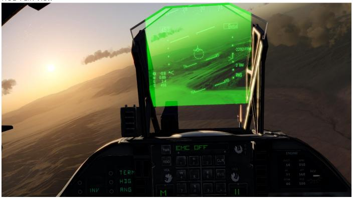
Selecting Night Mode on the HUD Control Panel enables HUD FLIR View. This mode shows Infra-red night vision video projected onto the HUD. Adjust video brightness and contrast with adjacent knobs.
