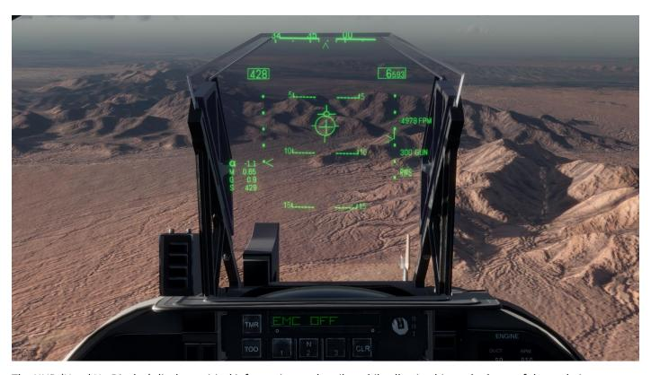
The HUD (Head Up Display) displays critical information to the pilot while allowing him to look out of the cockpit.
