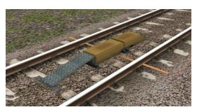
AWS is provided to give train drivers in-cab warnings of the approach to signals, reductions in permissible speed and temporary/emergency speed restrictions, and to apply the brakes in the event that a driver does not acknowledge cautionary warnings given by the system.
