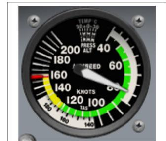
**Figure 2.11:** The airspeed indicator in the Cessna 172 [Full size →]
