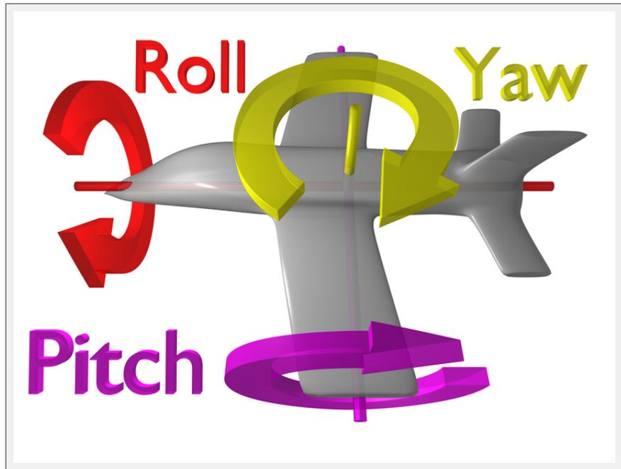
**Figure G.1:** The flight dynamics of an aircraft. Thanks to Wikipedia contributor ZeroOne for releasing the image under the Creative Commons Attribution 3.0 Unported license. [Full size →]
