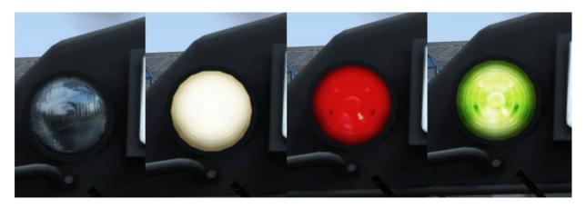
The P30CH is fitted with Classification lights. The purpose of these was to identify the train in accordance with the light in use.
